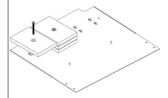
Each splice tray-mounting bracket is equipped with bolts. Remove these screws and slide one, two, or three Universal Splice Trays on to each bolt, depending on density required. Screwing the bolts back into the splice tray-mounting bracket secures the splice trays in place. Table 2 shows combination of screws for different Splice Kit.
