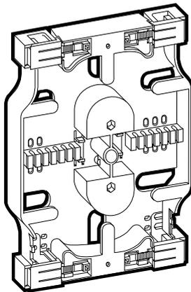
Splice Tray with Mechanical Splice Sleeves
