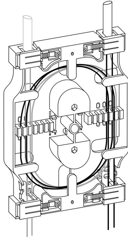
5. There is now enough fibre in the tray to make splices and leave at least one complete loop of fibre in tray. Proceed with the splices. Before each splice is done, determine which slot in the splice sleeve the finished splice will occupy and trim the fibre to the proper length.
