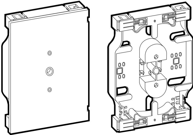
1. The Splice tray includes either two fusion splice sleeves or two mechanical splice sleeves. Install them into the splice tray as shown. The fusion splice sleeve snaps into position; the mechanical splice sleeve is adhesive-backed.
