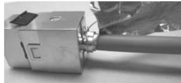
7c. Tighten the drain wire over the metal cable collar to maintain shield continuity.
