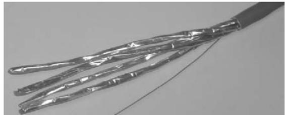
6c. Remove 3 of the 4 foils from the cable pairs. Unwrap the foil from 1 pair in preparation for wrapping around the cable sheath.
