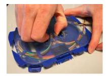
Place thumb and first finger in lid cutouts and flex lid up at center to release.
