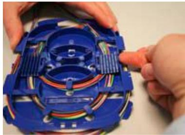
Use finger nail or tapered end of fiber pick on splice holder tab to lift and pivot upwards.
