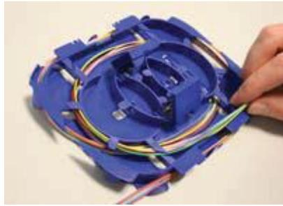
Routing underneath splice holder area
