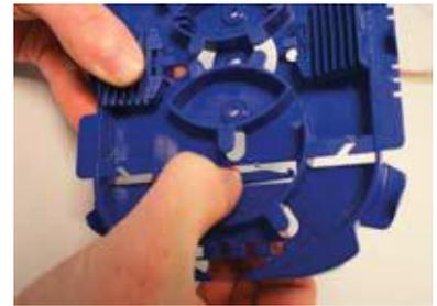
To remove fiber pick press down firmly on pick before mounting tray.
