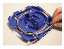
Routing underneath splice holder area
