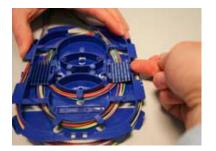
Use finger nail or tapered end of fiber pick on splice holder tab to lift and pivot upwards.
