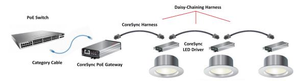
The total power budget on the Gateway must comply with the UPOE standard, and considers the load power, power drop on CoreSync devices in the Daisy-Chain–including the Gateway, and interconnect losses. The overall voltage drop and power drop can be calculated prior to the design. Please refer to CoreSync Harness Length Calculator to calculate the maximum run distance.
