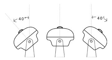
When used with the bracket mount, the sensor can be placed 40° one way, 40° the other way, or direct center.
