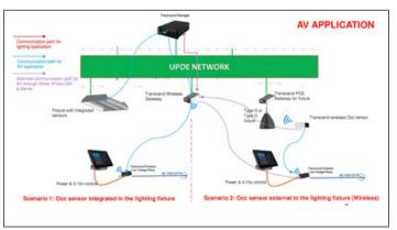
FIGURE 5: Diagram showing the connectivity and communication path for GP's AV application.
