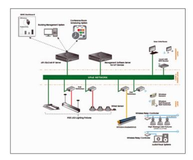
FIGURE 4:Network topology of GP's IoT and PoEenabled integrated platform.
