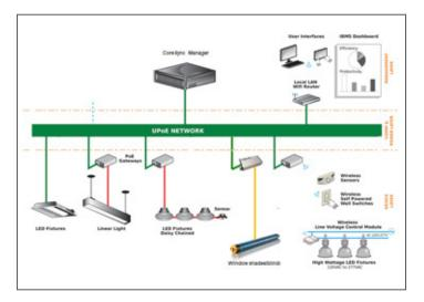
FIGURE 7: Network topology of GP's lighting platform.
