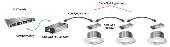
The total power budget on the Gateway must comply with the IEEE 802.3bt standard, and considers the load power, power drop on CoreSync devices in the Daisy-Chain–including the Gateway, and interconnect losses. The overall voltage drop and power drop can be calculated prior to the design. Please refer to CoreSync Harness Length Calculator to calculate the maximum run distance.
