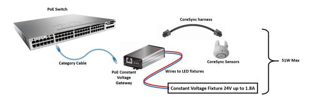
The total power budget on the Gateway must comply with the UPOE standard, and considers the constant voltage load power, power drop on CoreSync devices in the Daisy-Chain–including the Gateway, and interconnect losses. The overall voltage drop and power drop can be calculated prior to the design. Please refer to CoreSync Harness Length Calculator to calculate the maximum run distance.
