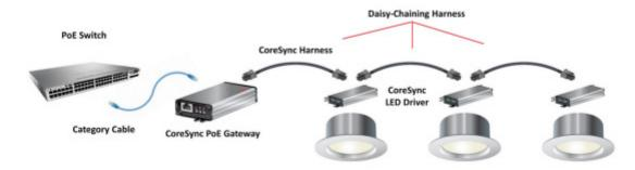
The total power budget on the Gateway must comply with the IEEE 802.3bt Standard, and considers the load power, power drop on CoreSync devices in the Daisy-Chain - including the Gateway, and interconnect losses. The pverall voltage drop and power drop can be calculated prior to the design. Please refer to the CoreSync Harness Length Calculator to calculate the maximum run distance.
