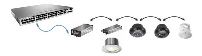
\* Minimum Guaranteed Power for Gateway 1.0 is 51W and Gateway 2.0 is 71.3W. The total power budget on the Gateway must comply with the requirement.
