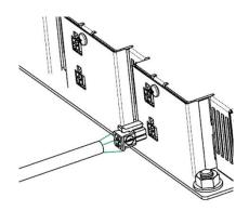
**Step 7.** On the front side of the unit, connect PoE CAT cable until you hear a "CLICK". Use a UTP (Unshielded Twisted Pair) CAT5E or CAT6 Cable.
