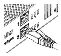
**Step 7.** Please Note that the Power LED indicator will turn on once you have the power. The Link and Active indicator will blink on and off rapidly once you have the network connection.
