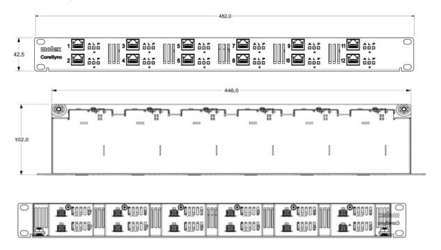
**Step 1.** Only to be installed with the standard 1U rack.
