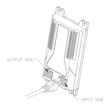
**Step 4.** Use #8 self-tapping screws to mount the Interface Module
